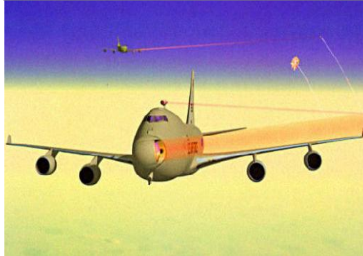
Figure 1. ABL v. ATL. The ATL (1a.) engages a target on the ground. The turret on the ATL is located underneath the aircraft. The ABL (1b.) flies above the lower troposphere and engages targets such as intercontinental ballistic missiles (ICBMs). The turret on the ABL is located on the nose of the aircraft. Courtesy of Popular Science Magazine and the United States Missile Defense Agency. http://www.popsci.com/scitech/article/2004-06/advanced-tactical-laser
